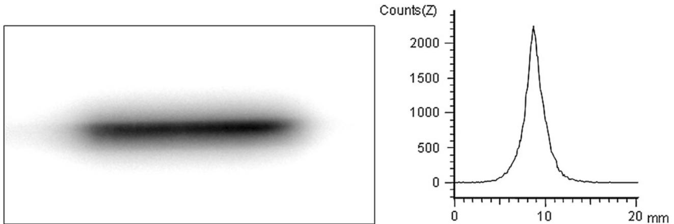
**Fig. 2** Re-188 filled balloon catheter: Energy distribution from a Re-188-filled balloon catheter as visualized by a Phosphor imager (PosphorImager SI, Molecular Dynamics GmbH, Krefeld, Germany).
